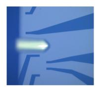
Cleaning of a photomask using a sharp robust diamond probe. A significant amount of debris is removed from the surface without damaging the photomask. Acquired using an Asylum Research Cypher-S AFM using an Adama Innovations Photo Mask probe.
