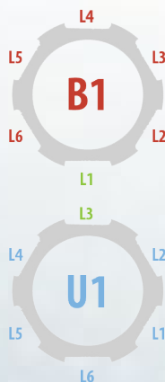
Figure 2. Fired Beretta bullets have six land impressions that are analysed to find a match in both form and sequence.
