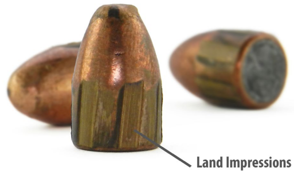
Figure 1. Impressions left on a Beretta bullet.
