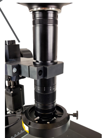
High quality 20X zoom lens, providing great quality images and flexibility, Can also be used with infinity-corrected objective lens.
