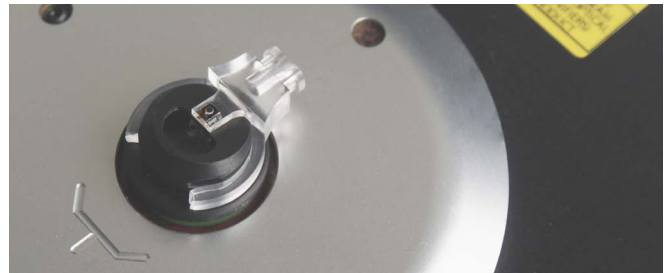
PERFECT INTEGRATION WITH YOUR INSTRUMENT. FluidFM® pipette mounted on AFM scan head.
