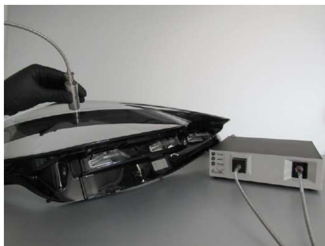
Characterization of a multi-layer stack on a lens for automotive lamp.
