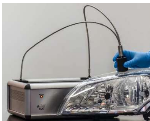
Characterization of a multi-layer stack on a lens for automotive lamp.
