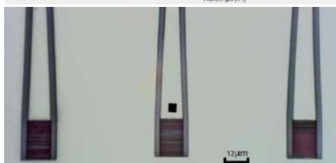
1520.6nm UV5 resist/202.2nm Si 3 N 4 /3090.7nm SiO 2 /Si, VIS/NIR tools
