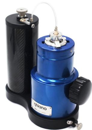
Tuning the pore size, applied pressure and voltage improves the measurement sensitivity and enables a wider range of particles to be analysed.
